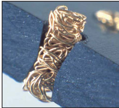
Connector Cross Section Showing CIN::APSE® Contact
